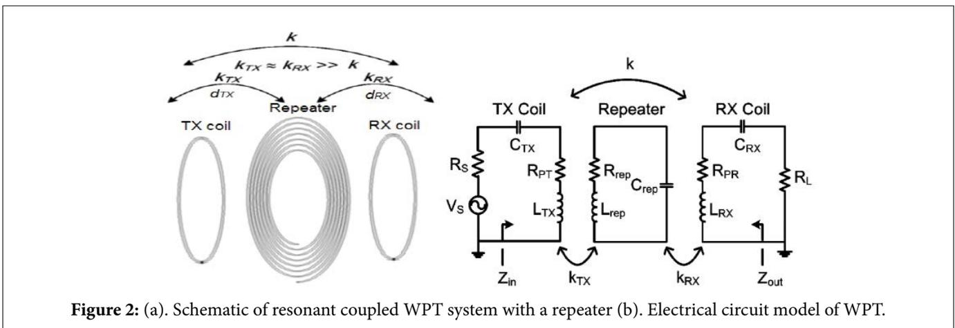
Figure 2: (a). Schematic of resonant coupled WPT system with a repeater (b). Electrical circuit model of WPT.
